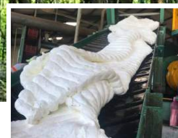
After removing impurities, formic acid helps to coagulate the sap into a workable consistency.
