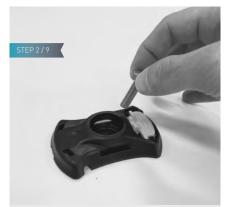
1. ASSEMBLY: Remove the big center screw from the base which comes with your iRIG.
