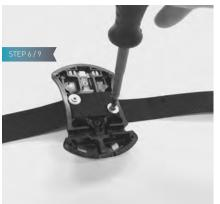
Now turn the base upside down, take a Philips-head screw-driver and fix the webbing to the base with 2 screws and washers.
