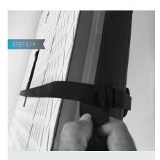
Thread the webbing through the buckle but do not fully tension it yet.
