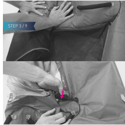
As soon as you have completely deflated the boom-bladder close the switch as indicated by the arrow.
